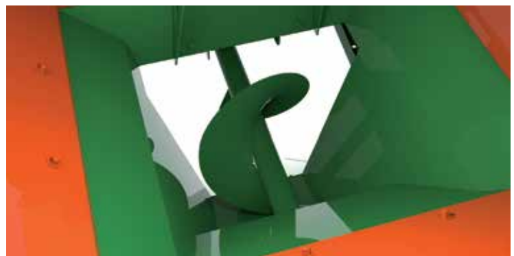
Uncovered auger as viewed from hopper above
